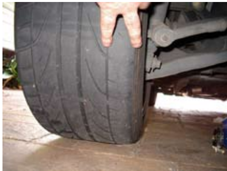
Bad Alignment = uneven tyre wear
